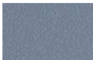
6 TEXTURE Rougher texture for better texture retention after forming and matte surface
